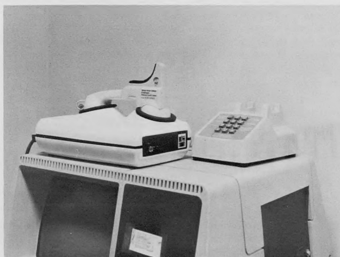
Figure 2: The telephone receiver as it rests on its coupler. This coupler is portable but in this case is sitting on the terminal.
