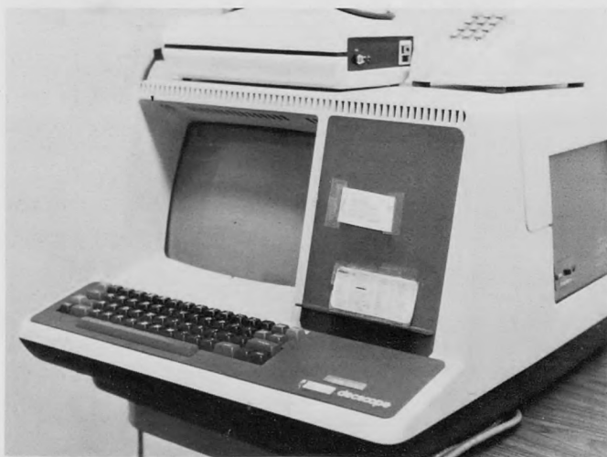
Figure 1: This terminal has a standard typewriter keyboard and has the capacity of presenting 12 lines of the computer program at any one time. Each line can contain up to 80 letters, punctuation marks, or numbers.
